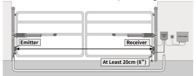
◆ Once the installation position is determined, drill mounting holes to match the holes on the sensors. Secure the sensors with the included screws. For better stability, it is recommended to place a rubber pad (not included) between the sensor and the mounting surface.
