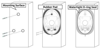
**Note:** Attach the included watertight O-ring seals to the sensors for waterproof protection.
