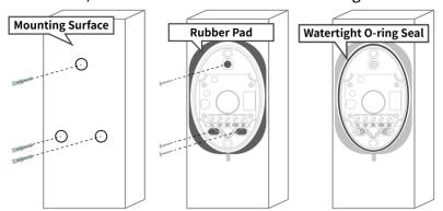
**Notes:** Attach the included watertight O-ring seals to the sensors for waterproof protection.
